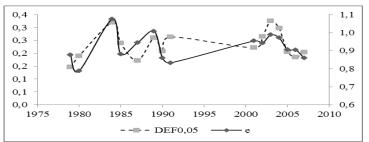
**Fig. 3 Diagram of changes of average values of the massif parameters in time. Notes:** e –the coefficient of porosity; DEF0, 05 –the absolute ground deformation of the natural moisture on the pressure level 0.05 MPa.
